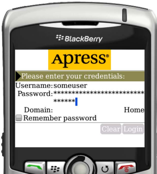
Figure 5-18. The labels are aligned on the right. Notice that wrapping is supported for the password field too.
