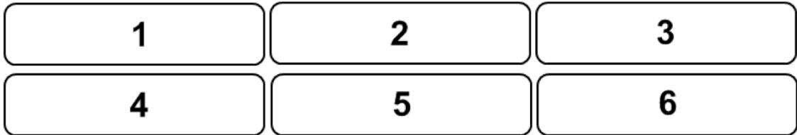
Figure 5-19. Grid manager with six fields. Fields number 2, 3, 5 and 6 are focusable.
