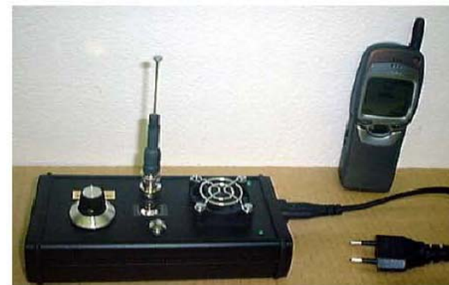
Low power room GSM jammer, (900/1800 Mhz)
