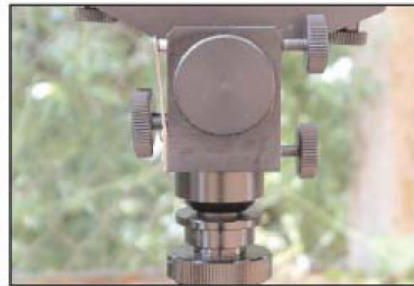
Close up of fine/coarse tripod adjustment
