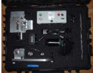
Powered drilling system
