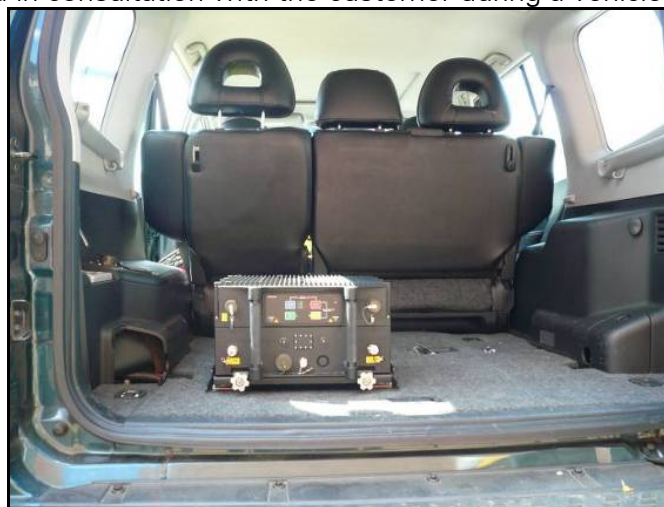
Figure 3-2: WBS2500 Unit Vehicle Installation
