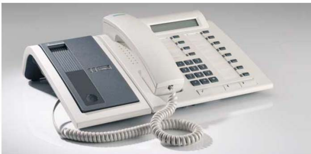
Optiset E privacy module with Optiset E telephone and support tray
