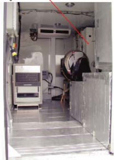
hoop module creates the "Flying Spot" X-ray. Backscatter detectors collect the reflected X-rays for image processing.
