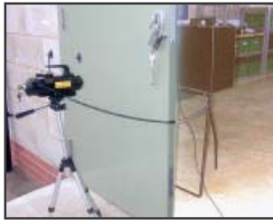
Use Model 7504 to search behind walls, doors or vehicle panels (hidden bug detection)
