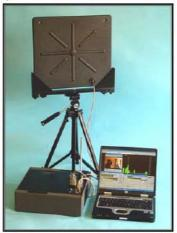
This is a portable system for radio frequency surveillance analysis. As a Far Field Counter Measure it can monitor a large area of many rooms or can target one at a time. It is easily programmable, with results stored for repeated and future appraisal, with a full A4 report printout of text and graphical display in line or bar. A novice user with a modest background in radio scanning can have the unit operational in 30 minutes to produce a fully documented predetermined scan.
