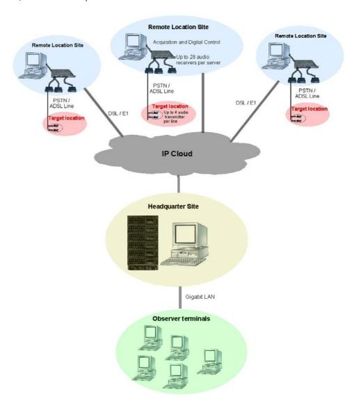
Audio is captured form a target location by audio transmitters containing tiny microphones, and transferred to the remote location site over a telephone line. Usually, a remote location site exists near a location exchange. It contains a large bank of receivers to collect audio from various target locations. The received audio channels are digitized and stored in a remote location server.
