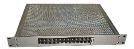
ACQ uses four 8-bit analog to digital converters to digitize the audio channels. The digital audio samples are buffered before sending them to XRLS-SER using a USB 2.0 interface. Main features of the XRLS-ACQ platform are listed below:
