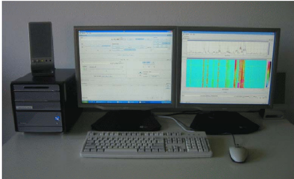
Exemplary workstation configuration comprising of PC, two TFT-displays and an active loudspeaker box.
