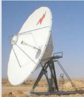
Example for SAT-dish for monitoring the up and down link between Satellite and gateway (approx. 10mtr)
