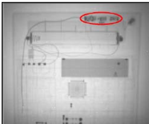
X-ray view of calculator and pen with inbuilt transmitter
