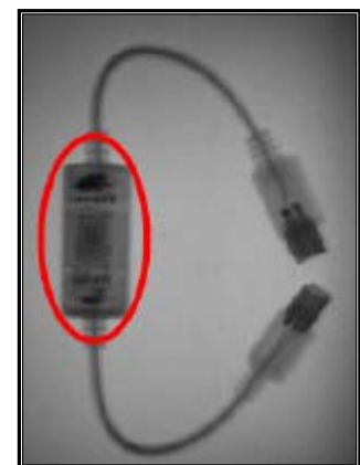
Keyboard connector with concealed logger
