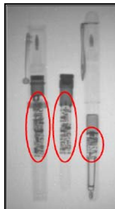
X-ray view of calculator and pen with inbuilt transmitter
