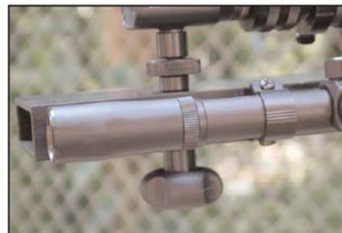
4 x 20 Finder Scope with cross hair mounted on Picatinny rail (rail fitted to both sides).
