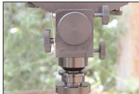
Close up of fine/coarse tripod adjustment
