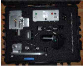
Powered drilling system
