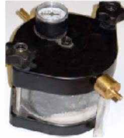
Vacuum & spoil extraction system
