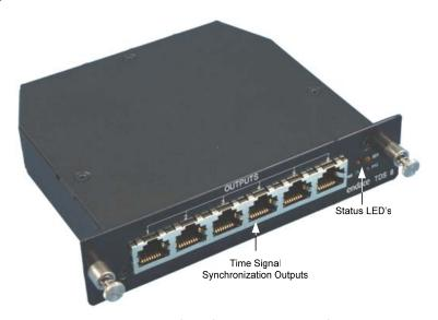
A TDS6 Expansion unit connects to the Chain output on the TDS2 Server Module. The synchronized time signals travel from the TDS2 Chain port to TDS6 expansion units through chain cables. The signals travel to DAG cards via the TDS6 Expansion unit synchronization outputs.
