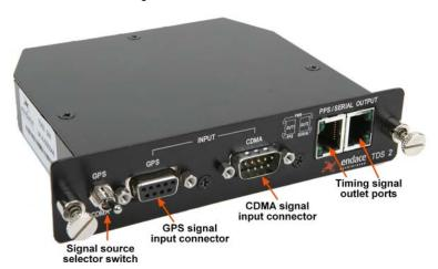
The time synchronization outputs use RJ45 connectors and can be connected to the time synchronization sockets on the front bracket of a DAG card using standard Ethernet cables and patch equipment.
