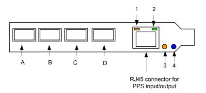
When a DAG 4.5G24 series card is powered up the LED 1 should always come on.
