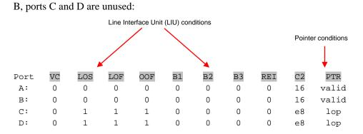
In the example below the card is set to OC-3 PoS while the line carries OC-12 PoS:
