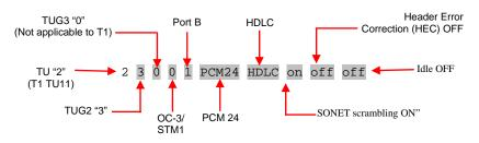
This configuration is shown in the <u>*T1 OC-3/STM-1*</u> diagram in <u>*Valid*</u> <u>*Configurations*</u> earlier in this chapter.
