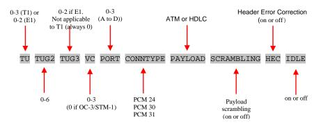
In the example line below the channel is configured for E1 channelised OC-3/STM-1, port A containing ATM over PCM-30.
