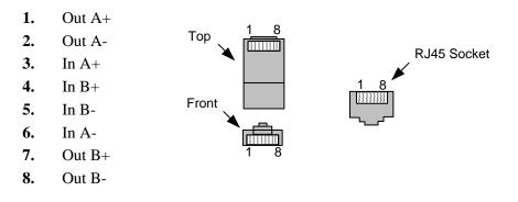
Normally you should connect the GPS input to the A channel input (pins 3 and 6).
