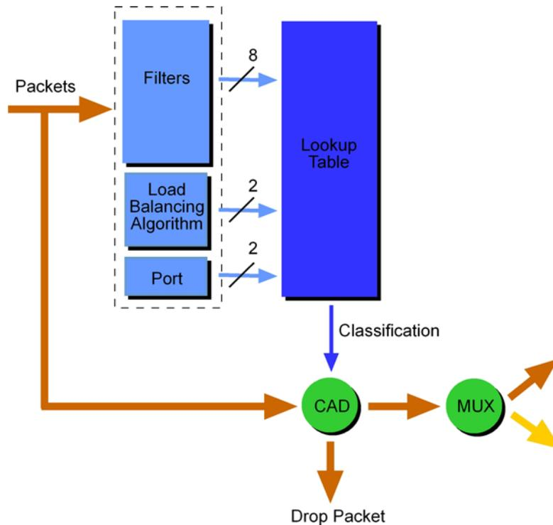
Packets are received from the line and stamped with an ERF (Endace Record Format) header, then pass along to the filter and load balancing block.
