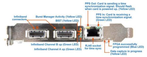
There is an 8-pin RJ-45 socket located near the InfiniBand connectors which is available for connection to an external time synchronization source.
