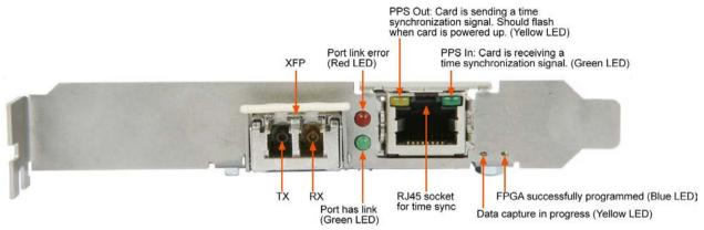
There is an 8-pin RJ-45 socket located below the XFP connector which is available for connection to an external time synchronization source.
