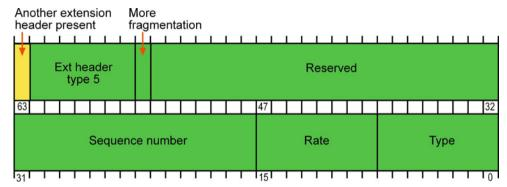
The following details the make up of the <code>Raw\_Link</code> Extension Header:
