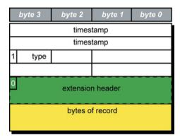
The following diagram shows presence of two Extension Headers with Bit 7 of the first Extension Header set to '1'.
