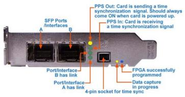
**Note:** The DAG 7.5G2 supports both optical and copper transceivers.
