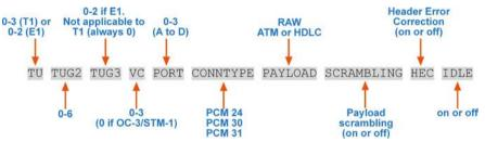
In the example line below the channel is configured for E1 channelized OC-3/STM-1, port A containing ATM over PCM-30.
