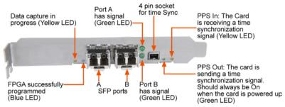
In addition there is a 4-pin socket located beside the port connectors which is available for connection to an external time synchronization source.
