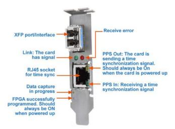
There is also an 8-pin RJ45 socket located beside the XFP connector which is available for connection to an external time synchronization source.
