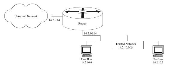
Figure 5-1: A Simple Router Firewall
