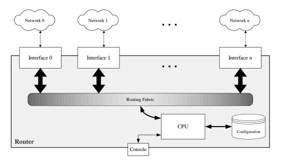
Figure 2-4: A Notional Router's Hardware
