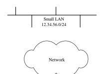
A local-area network (LAN) segment, such as an Ethernet, is represented by a horizontal or vertical bus, with several connections.
