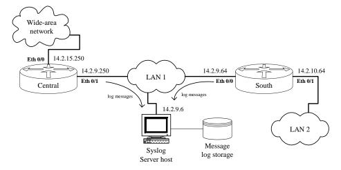
Figure 4-7: A Small Syslog Configuration
