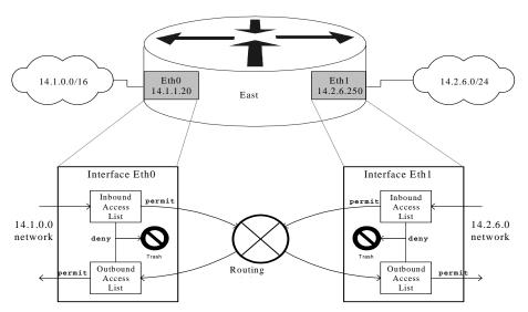
Figure 4-2: Conceptual Model for Access Lists on Interfaces
