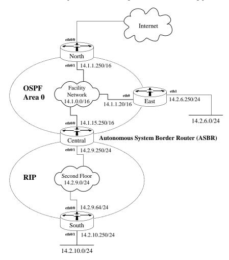
Figure 4-3: A Simple OSPF Routing Architecture
