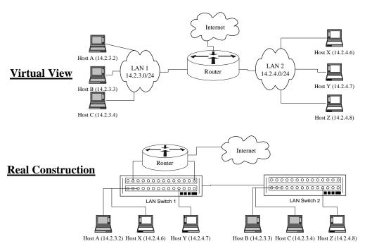
Figure 7-1: Virtual LAN Switching
