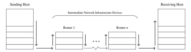
Figure 2-2: Moving Data through Protocol Stacks
