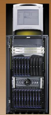
Example: 4000 channels, with storage and fax/data demodulation in 24 U rack
