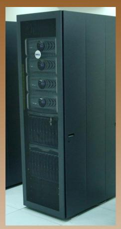
Capacity of more than 9000 channels and 160 TB in 1 rack, including fax and data demodulation. Remote gateways.
