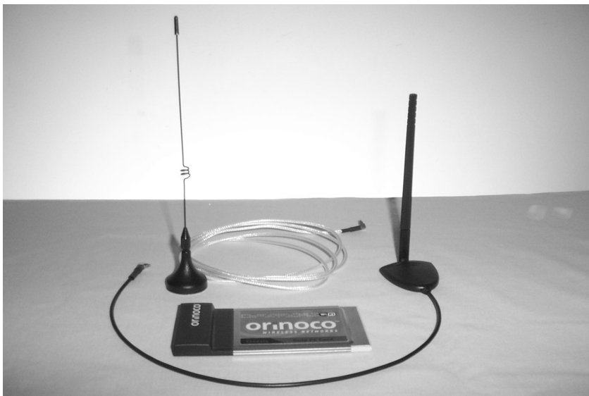
Figure 2.5 Small Omnidirectional Antennas - 5 dBi Gain
