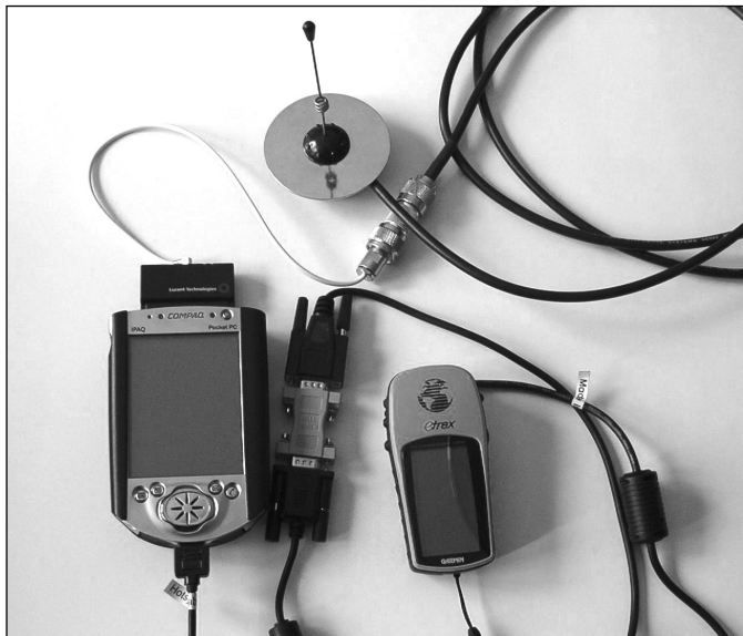
Figure 1.2 Typical PDA WarDriving Setup
