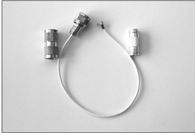
Figure 1.7 Pigtail for Use with ORiNOCO Cards and N-Type Barrel Connectors
