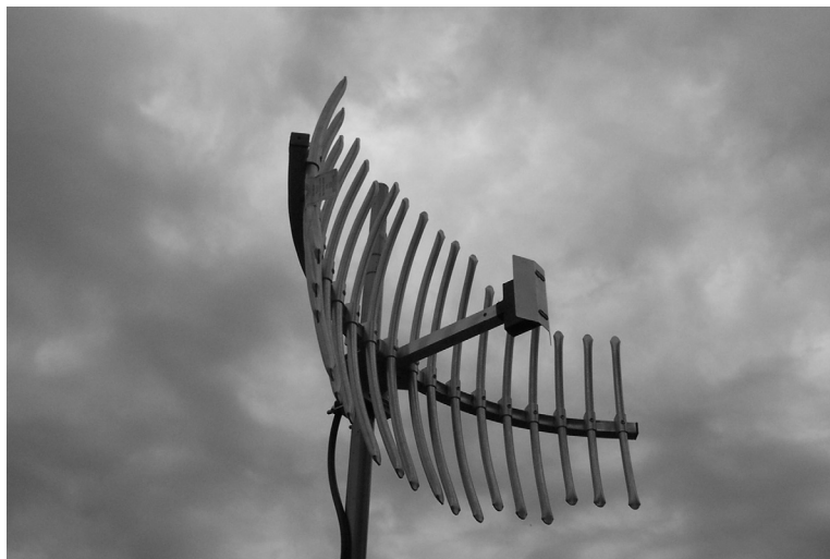
Figure 2.10 A Grid-type Directional Antenna
