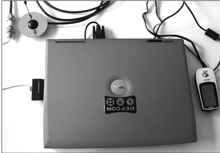
Figure 1.1 Typical Laptop Computer WarDriving Setup
