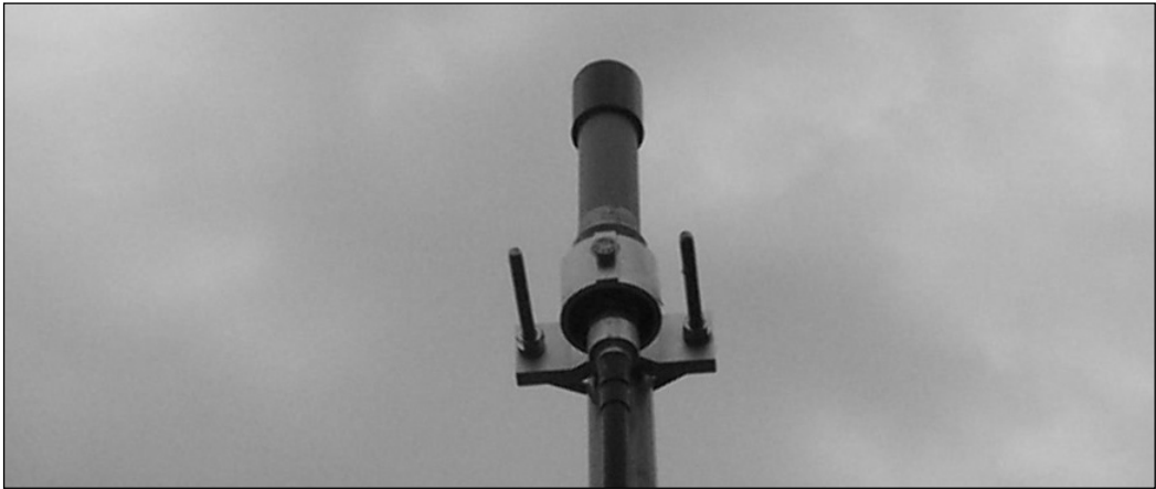
Figure 2.6 Mast-mounted Omnidirectional Antenna - 4.5 dBi Gain
