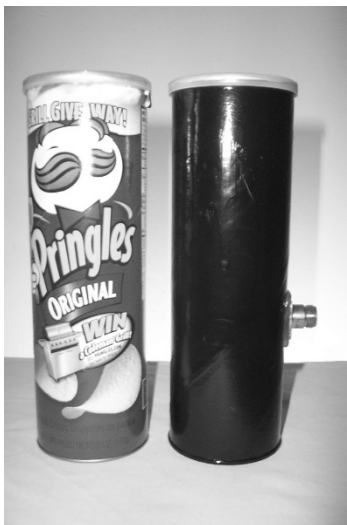
Figure 2.12 A Pringles can and finished Pringle’s “Cantenna”
