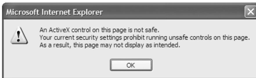
Figure 4.11. Setting Initialize and Script ActiveX Controls Not Marked as Safe to Disable prevents Internet Explorer from activating potentially dangerous ActiveX controls.
