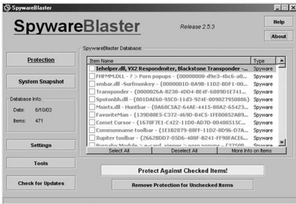
Figure 4.21. SpywareBlaster can set the kill bit for malicious ActiveX controls to prevent Internet Explorer from activating them.
