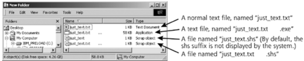
Figure 6.1. Hiding the EXE extension after several spaces.
