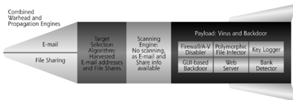
Figure 9.10. The Bugbear.B combo malware: A worm, virus, and backdoor combination.
