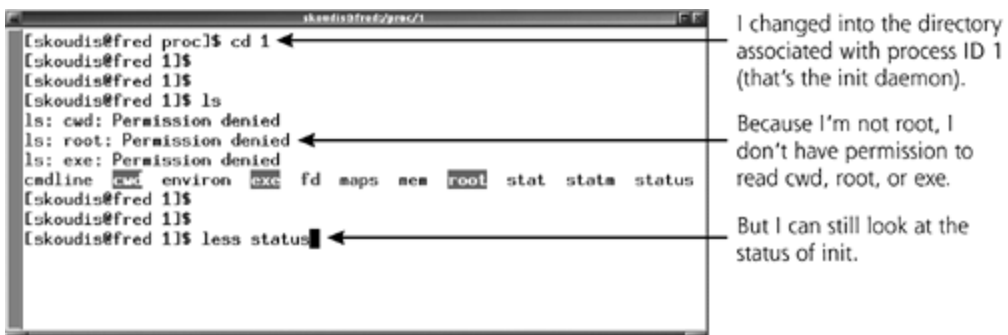
Figure 8.4. Looking inside a process ID in /proc to view its status.
