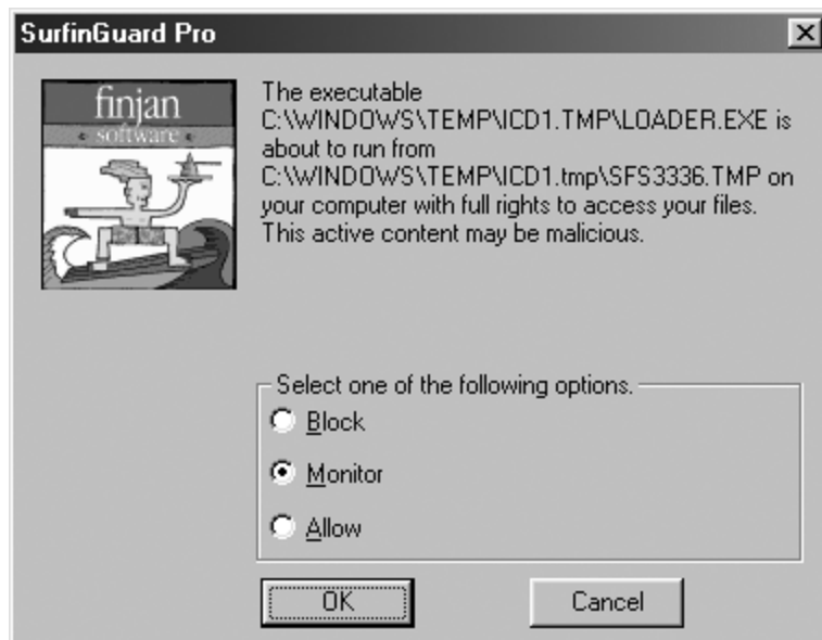
Figure 4.18. SurfinGuard can intercept and block actions taken by suspicious executables.
