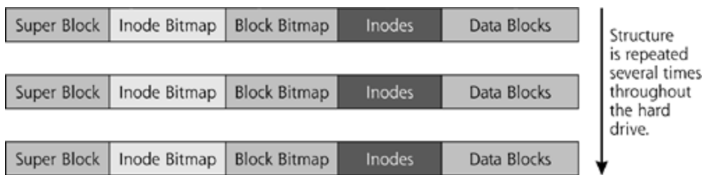
Figure 7.7. The organizing scheme of the ext2 file system brings together the super block, inode and block bitmaps, the inodes themselves, and data blocks.
