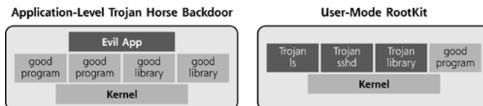
Figure 7.1. Application-level Trojan horse backdoors and user-mode RootKits.
