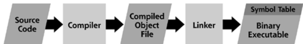
Figure 11.6. Going from source code to binary executable.
